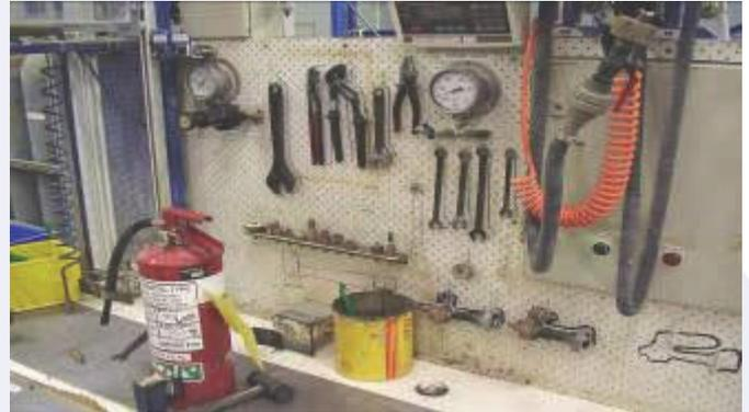
*Above: A "Shadow Board" is a very simple technique to slash "looking time" provided it is maintained.*
