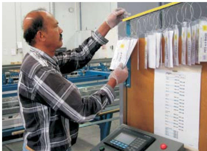
A machine operator at a TXM customer takes the Kanban cards from the rail in batches of four. Photos: TXM
