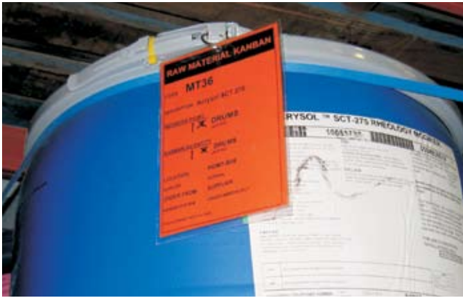
This is a variation on a Two Bin System at a TXM customer. When this drum is opened the Kanban card will be sent to purchasing who will order another drum to replace it.
